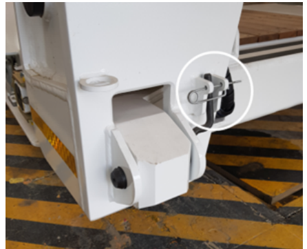
Pulling the safety pin
