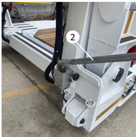
As a pump handle (2) when using the emergency hand pump
