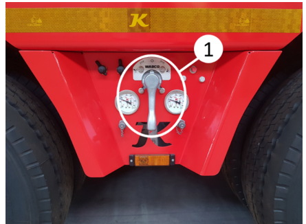
Manually operated air suspension driving position
