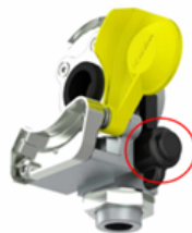
Palm coupling with a test point
