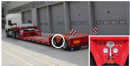
The location of the lowering / lifting valve
