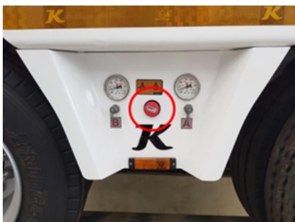
Parking brake control panel
