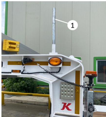
As a handle when climbing a gooseneck (1)
