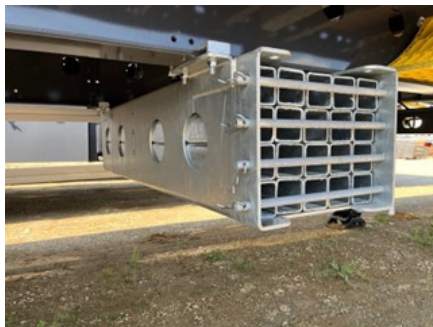
Under chassis pillar storage
