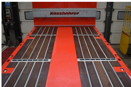
Hardwood floor with omega profiles
