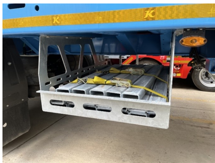
Under chassis pillar storage
