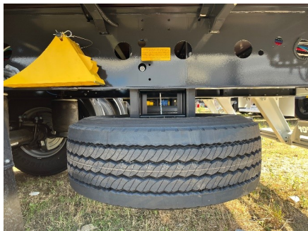
Rope type spare wheel holder
