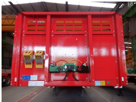
Wheel chock on front panel
