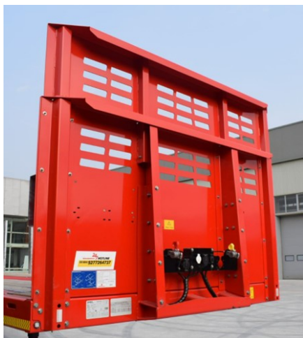
Bolted front panel
