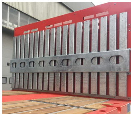
Pillar storage on front panel
