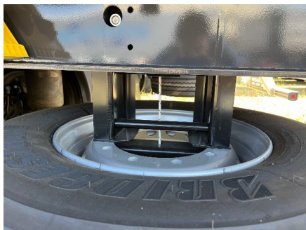
Rope type spare wheel holder
