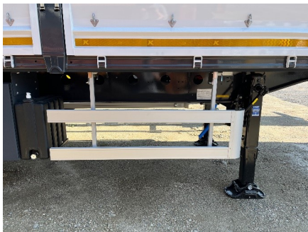
Side Underrun Protection
