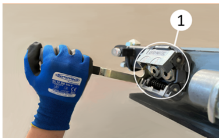
Duomatic Coupling Connection
