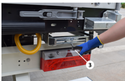
Foldable sliding ladder, removing the pin
