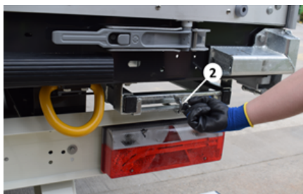
Foldable sliding ladder, removing the pin
