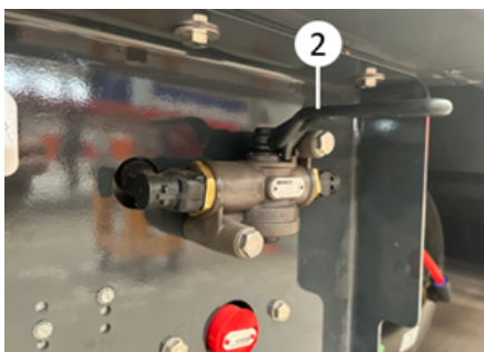
The Self Steering Axles Release Valve
